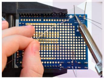
Solder in all the legs of the LEDs and resistors.
