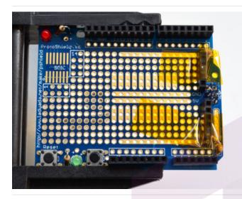
Place the two non-stacking 5-pin headers into the matching slots on the right hand side of the PCB. Use tape to keep them in place
