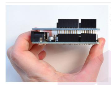
Now carefully plug the unsoldered headers into a spare Arduino. Make sure all of the long pins plug into the sockets on the side of the Arduino. There will be a gap between the shield and Arduino and the Printed Circuit Board will be loose
