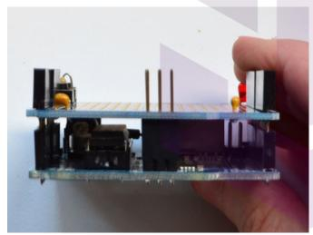
Plug the shield on top so that the 6 pins go through the matching holes in the PCB
