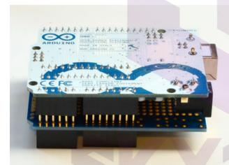
Flip over the Arduino and place it flat on the table so that the PCB sits flat against the stacky headers and the stacky headers are flat against the table
