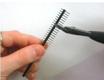
Next its time to make the male headers from the long strip. use diagonal cutters or pliers to clip off 4 parts, one 6-pin, two 8-pin, and one 10-pin
