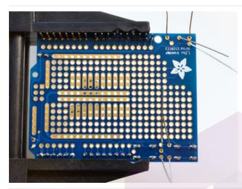
Bend out the leads of the LEDs and resistors so they sit flat againt the PCB
