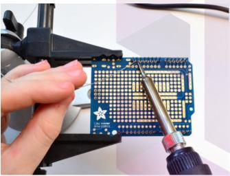
Now that you have aligned the stacky headers using an Arduino it's easy to finish the job
