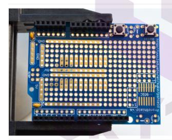
Snap the two buttons into the top corner of the PCB. They will snap into place and sit flat against the PCB. They are symmetric so you can insert them 'either way'
