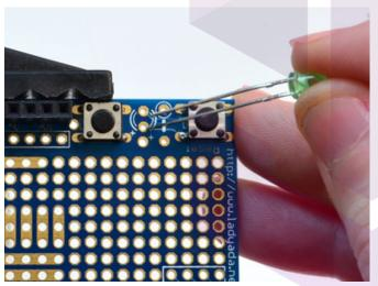
Next insert the small green LED between the two buttons. Like the red LED, check for the tiny + symbol on the PCB, aand place the longer leg of the LED into this pad.
