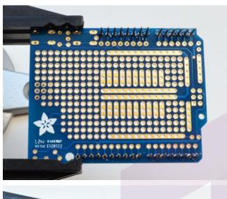
When done, check your work, make sure each pin is soldered with a nice shiny solder connection
