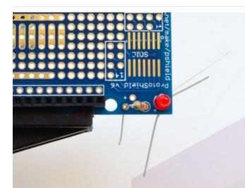
Next to the red LED you can bend one of the 1K ohm resistors over and insert it in the O- shaped silkscreen pads to the left
